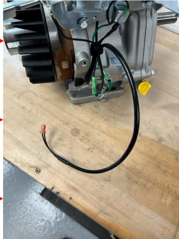
Pull wires from the carburetor to the back of the engine carefully
