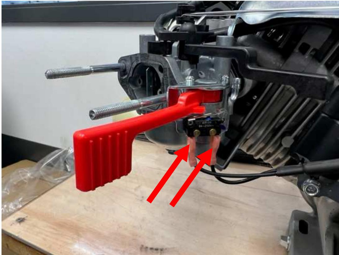
Disconnect the two wires from the switch at the Carburetor
