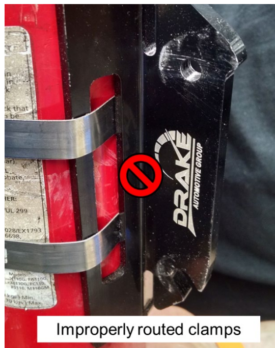
Figure B-52: Incorrect routing of hose clamps.
