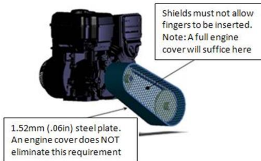
Figure B-43: Powertrain Guard Example
