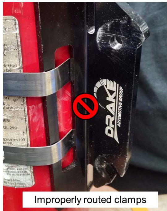
Figure B-47: Incorrect routing of hose clamps.
