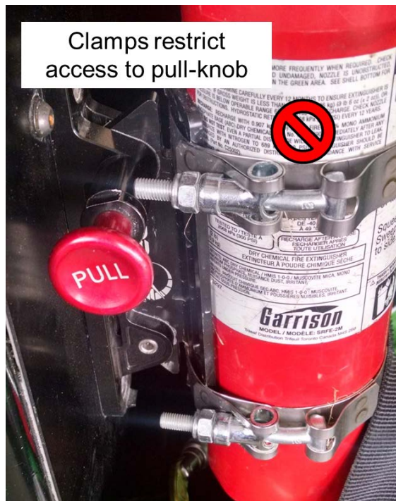
Figure B-46: Incorrect orientation of extinguisher clamps.
