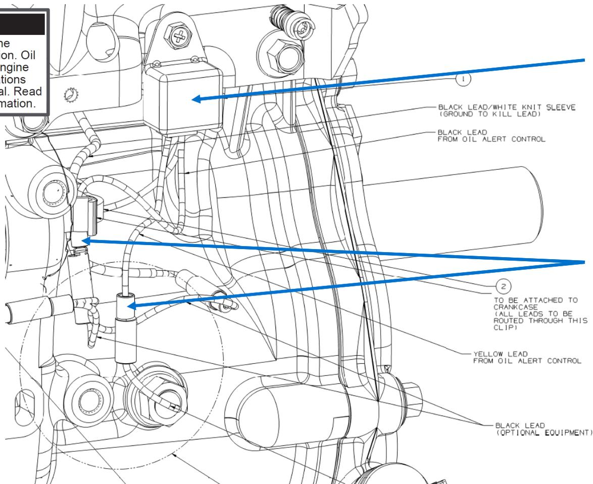
Remove Wiring and control module from the engine
