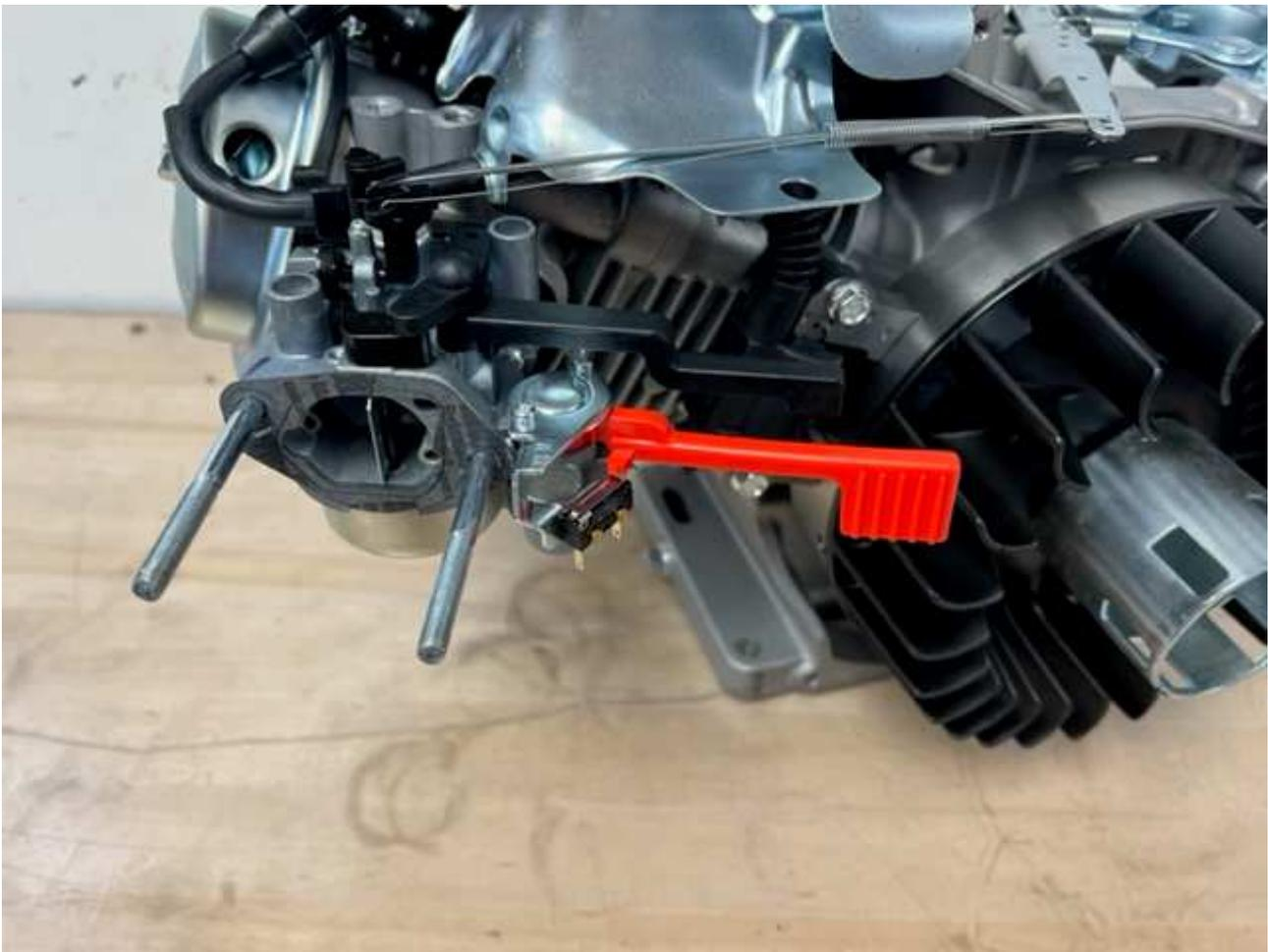
With this modification, the Red lever will not shutdown engine via spark but it will turn off fuel flow to the carburetor.
