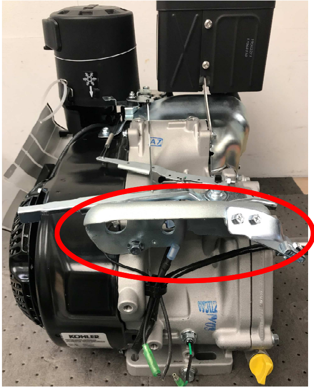
Fuel Tank Mount High Speed Setting Bracket PN 17 126 245
