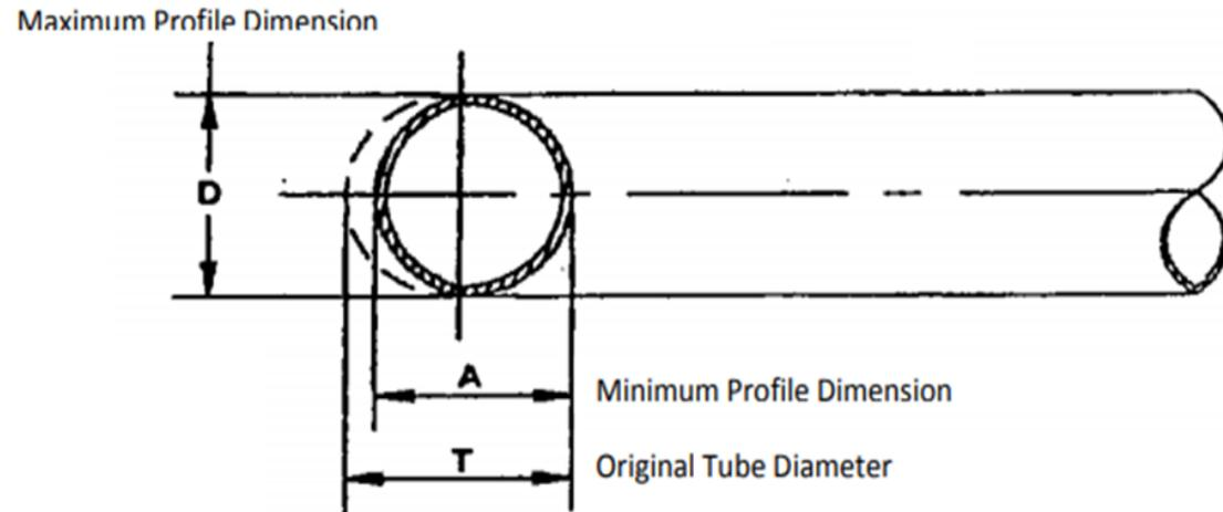
**Possible Solution:** Use a larger bend radius. CLR should exceed 4x the tube OD.
